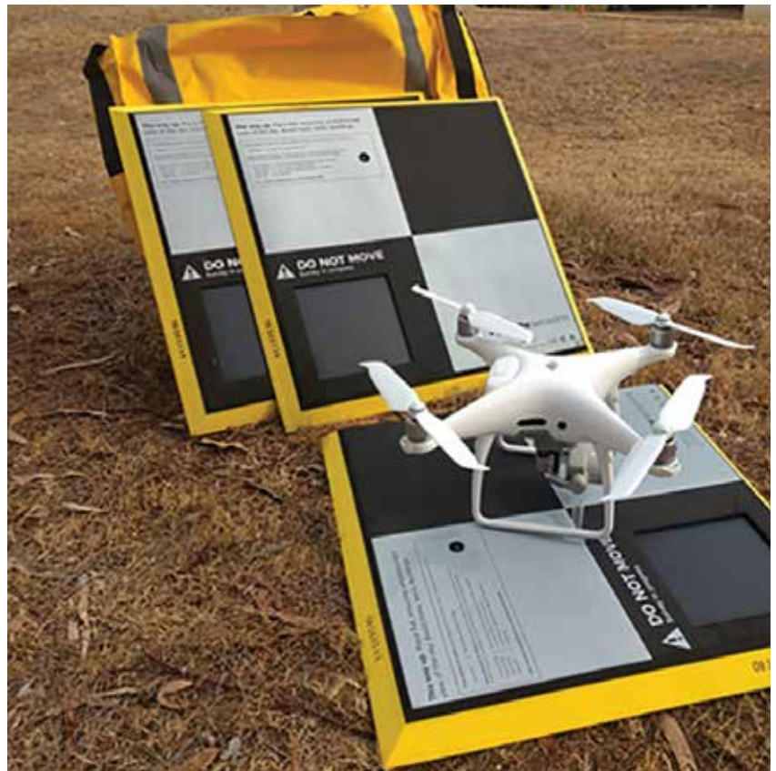
Photo 1: The drone with a high resolution camera and ground control points with accurate GPS locations are necessary to accurately measure pasture height.
