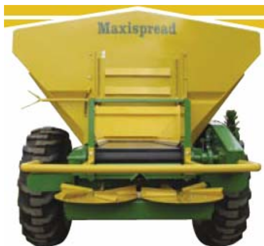
Photo 2. Horizontal flat spinners are also effective in spreading over a wide area. Landaco Maxispread. www.landaco.com.au
